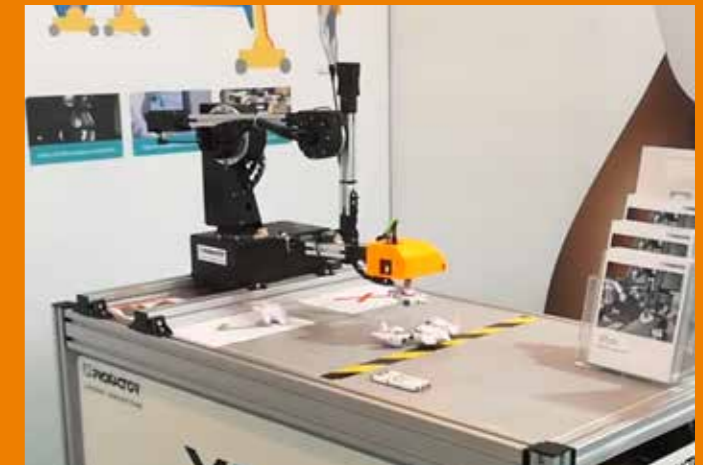
Measuring machine with RL-DQ-RBT-5532S and CPR control system for sorting good from bad parts (PROFACTOR GmbH)
