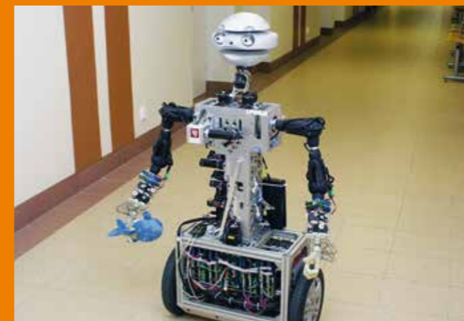
The Technical University at Wroclaw, Poland equipped its autonomous robot FLASH with 2 roboLink® articulated arms, each with 4 DOF.
