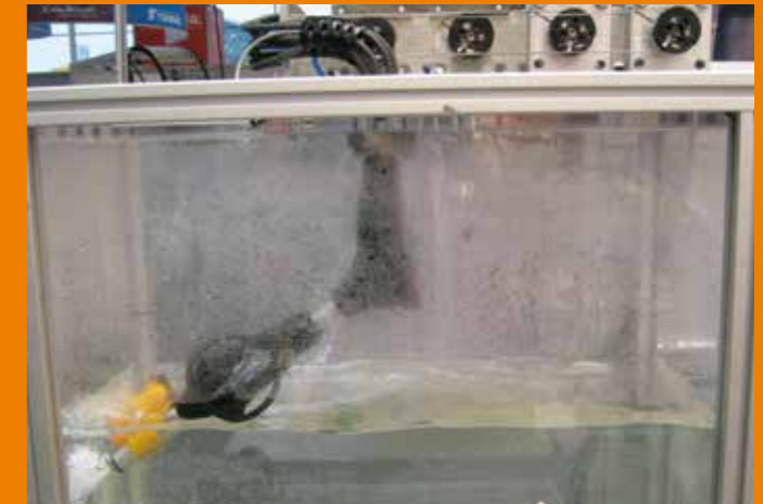
Submerged camera guidance, articulated arm with 4 DOF (igus®)
