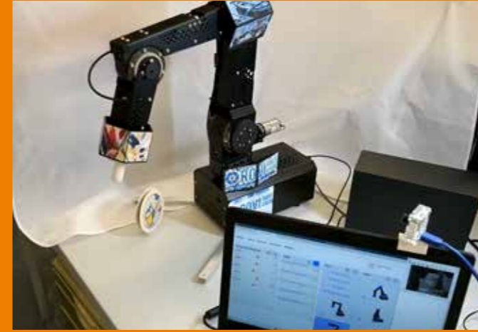
Camera-based control of a sensorless RL-D arm with 5 DOF (RoVi Robot Vision, TU Munich, LMT)
