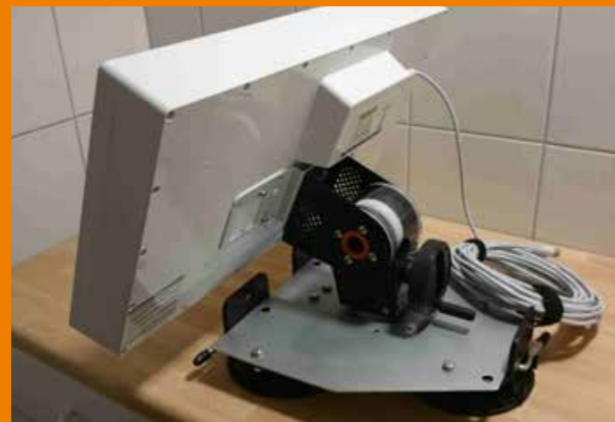
Manual adjustment of a receiver unit for satellite signals
