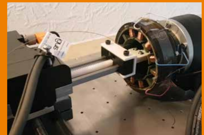
Winding machine prototype for BLDC motors with robolink® and drylin® components (Commonplace Robotics)
