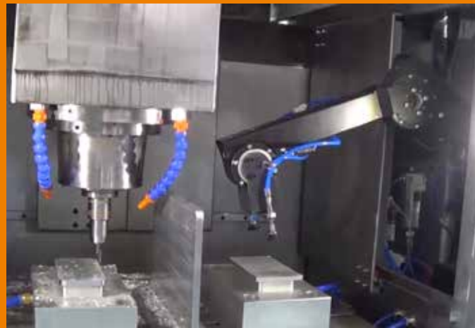
robolink® D – Suction arm in a machine tool (igus®)
