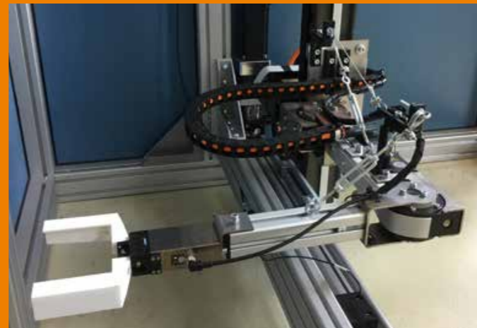
Storage and retrieval unit with two RL-D and drylin® linear guides (MATRIUM GmbH)
