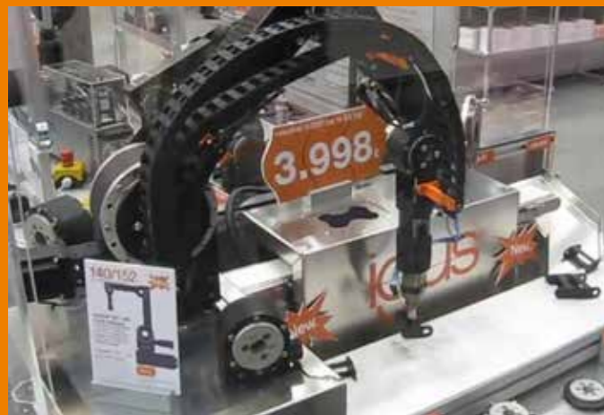
Trade fair machine – 5 DOF robot arm with RL-D and RL-S joints. System simulates real use in the igus® factory (igus®)
