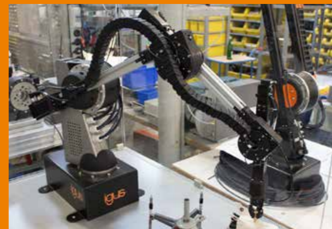
Trade fair machine RL-DQ-RBT-5532S-AC with 5 DOF and 3-finger gripper (igus®)
