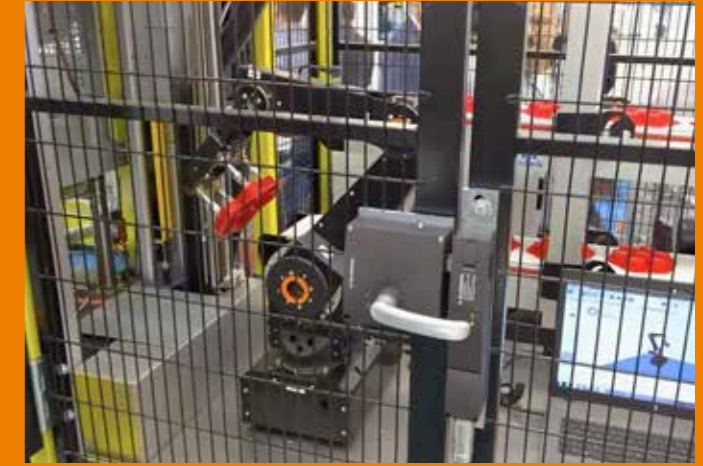
Injection-moulding process with automated handling thanks to robolink® D with 4 DOF (Dr. BOY GmbH & Co. KG)
