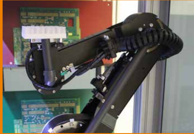
robolink® D for checking printed circuit boards (4Stars Engineering Systems GmbH)
